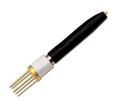
The FORX Photoreceiver is designed for high-speed and high sensitivity analog and digital applications, featuring a high bandwidth PIN photodiode and a linear preamplifier within a hermetically sealed coaxial package. The module incorporates a highly stable optical coupling system. Its low input-referred noise ensure exceptional linearity and precision.
